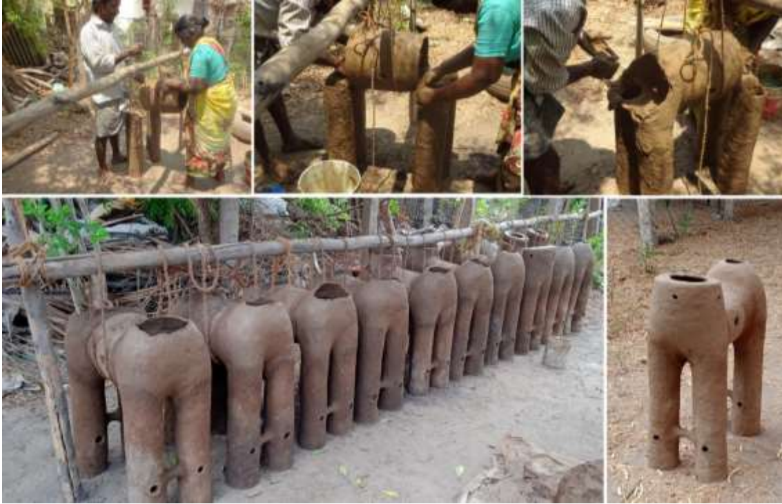
Figure 9: Attaching the Body and Legs
