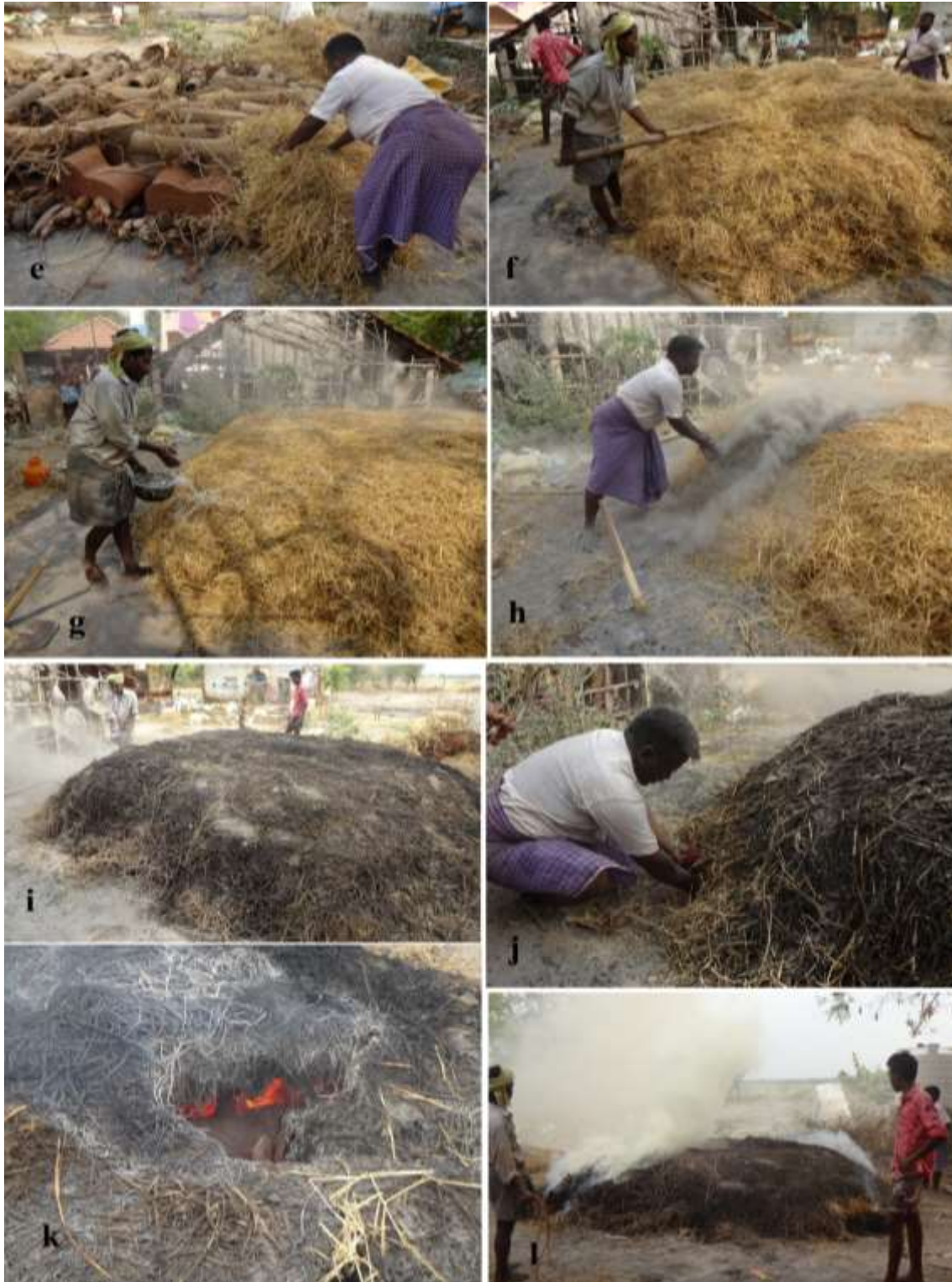
Figure 12: e) Placing rice straw on top of the terracotta horse, f) Arranging the rice straw over the terracotta horse, g) Sprinkling water on the terracotta horse, h) Covering the terracotta horse with ash and sand, i) Fully covered terracotta horse, j) Igniting the fire at the bottom, k) The terracotta horse being heated in an open kiln, and l) the firing process of the terracotta horse.
