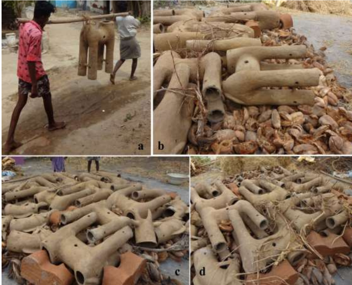
Figure 11: a) Carrying the terracotta horse to the open firing area, b) Coconut husk spread at the bottom of the firing setup, c) Complete arrangement of the terracotta horses for the firing process, and d) Small wooden pieces placed on top of the terracotta horses.
