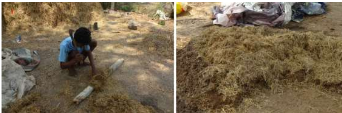
Figure 1: a) Chopping the rice straw; b) mixing the clay with rice straw
