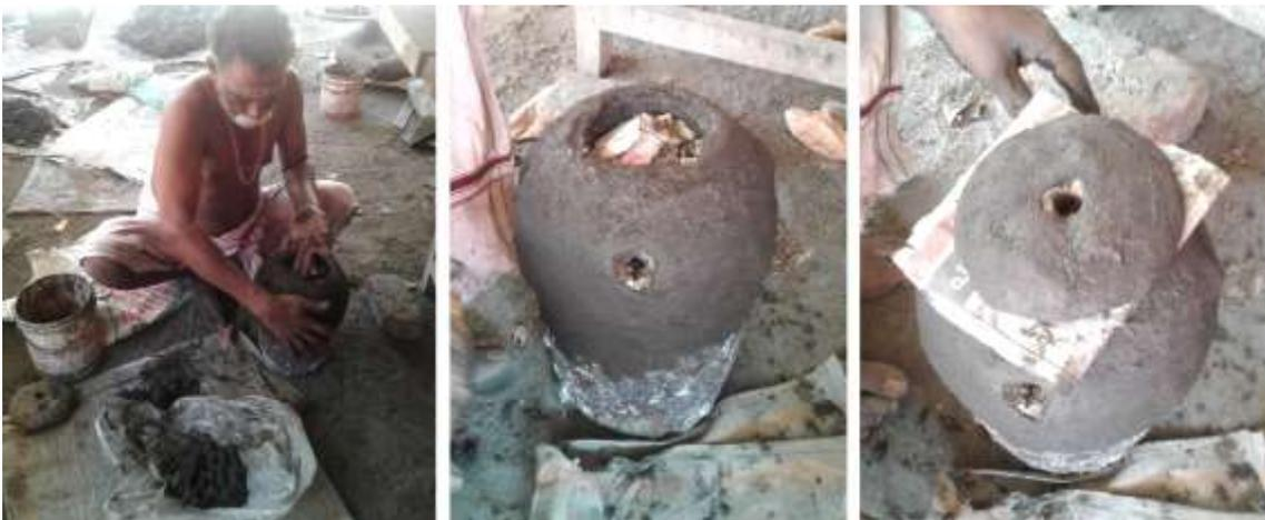
Figure 12: Crucible Preparation
