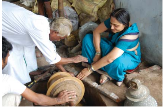
Fig. 10: Making of mould for bell casting at Nacharkoil, Tamil Nadu (Bell maker late Govindrajan with Sharada Srinivasan)
