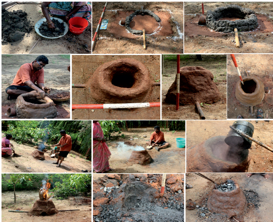
Fig. 11: 2 nd Phase of Iron Smelting Processes
