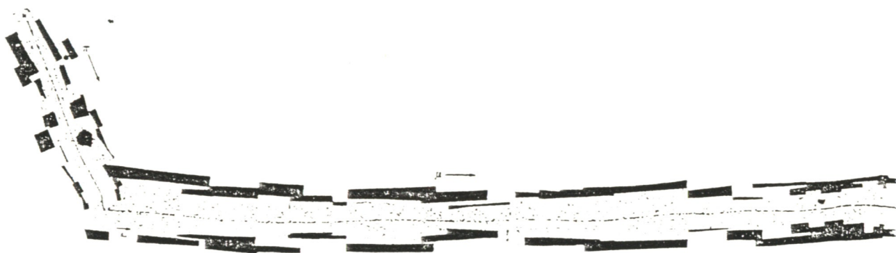
Photomicrograph showing a \pi meson ( \pi ) coming to rest in a nuclear emulsion and a \mu meson ( \mu ) arising from the end of the \pi -meson track. (From C. M. G. Lattes, H. Muirhead, G. Occhialini, and C. F. Powell, Nature , vol. 160, p. 453, 1947.)
