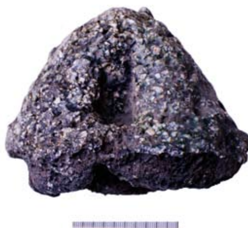
Fig. 8 Example of large, conical crucible lid showing indentations caused by the tongs used to remove the crucible from the furnace
